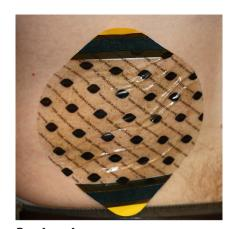
**Sand environment test**Image shows application with 2.9 g of sand applied to dressing to simulate application in desert environment.
